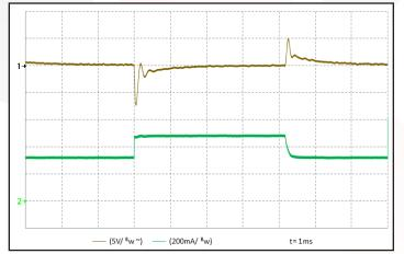
**Figure 11:** Output voltage response to step-change in load current (50%-75%-50% of Iout(max);  $dI/dt = 0.1 A/\mu s$ ). Load cap: 0.3  $\mu$ F ceramic capacitor. Ch 1: Vout (5 V/div), Ch 2: Iout (200 mA/div).(1 ms/div)
