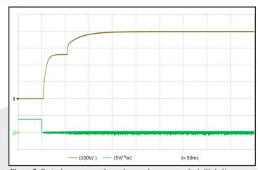
Figure 7: Typical startup waveform. Input voltage pre-applied. Ch 1: Vout (100V/div). Ch 2: ON/OFF (5V/div). (50 ms/div).
