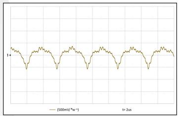
**Figure 10:** Output voltage ripple, Vout, at nominal input voltage and rated load current (500 mV/div). Load capacitance:  $0.3\mu$ F ceramic capacitor (2 $\mu$ s/div). Bandwidth: 10 MHz. See Figure 13.
