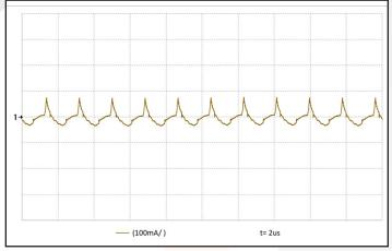
**Figure 9:** Input terminal current ripple,  $i_c$ , at full rated output current and nominal input voltage with 10µH source impedance and 4.7µF electrolytic capacitor (100 mA/div). (2µs/div) Bandwidth: 20MHz. See Figure 13.
