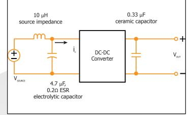
Figure 13: Test set-up diagram showing measurement points for Input Terminal Ripple Current (Figure 9) and Output Voltage Ripple (Figure 10).
